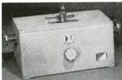
The standing-wave detector, a device for exploring energy distribution in a waveguide.
