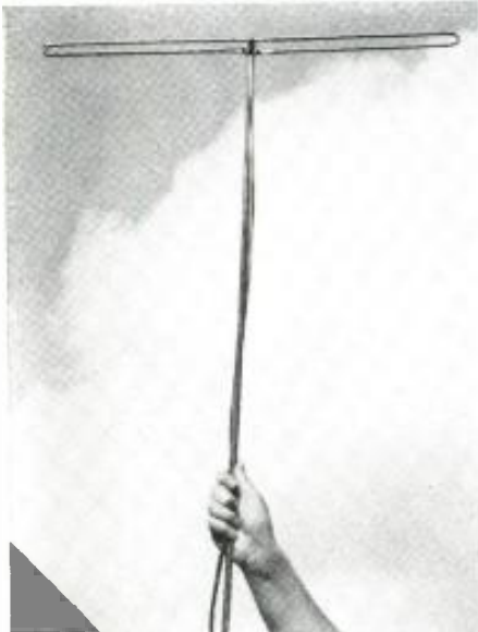
Fig. 4—Hand-held antenna used for testing.
